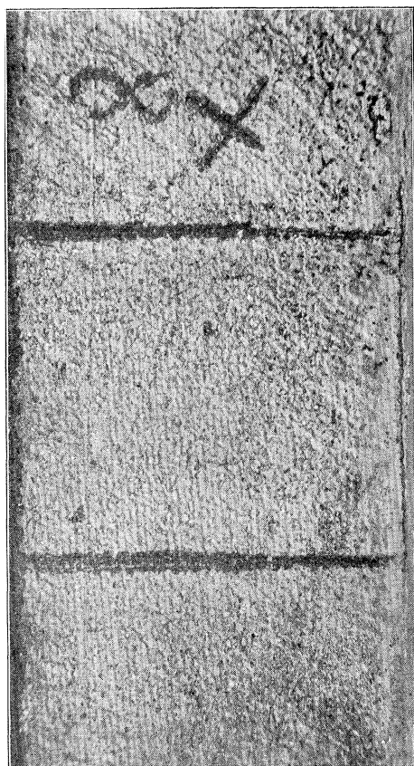
Fig. 15. A single crystal after straining in tension and re-etching \times 5 .
