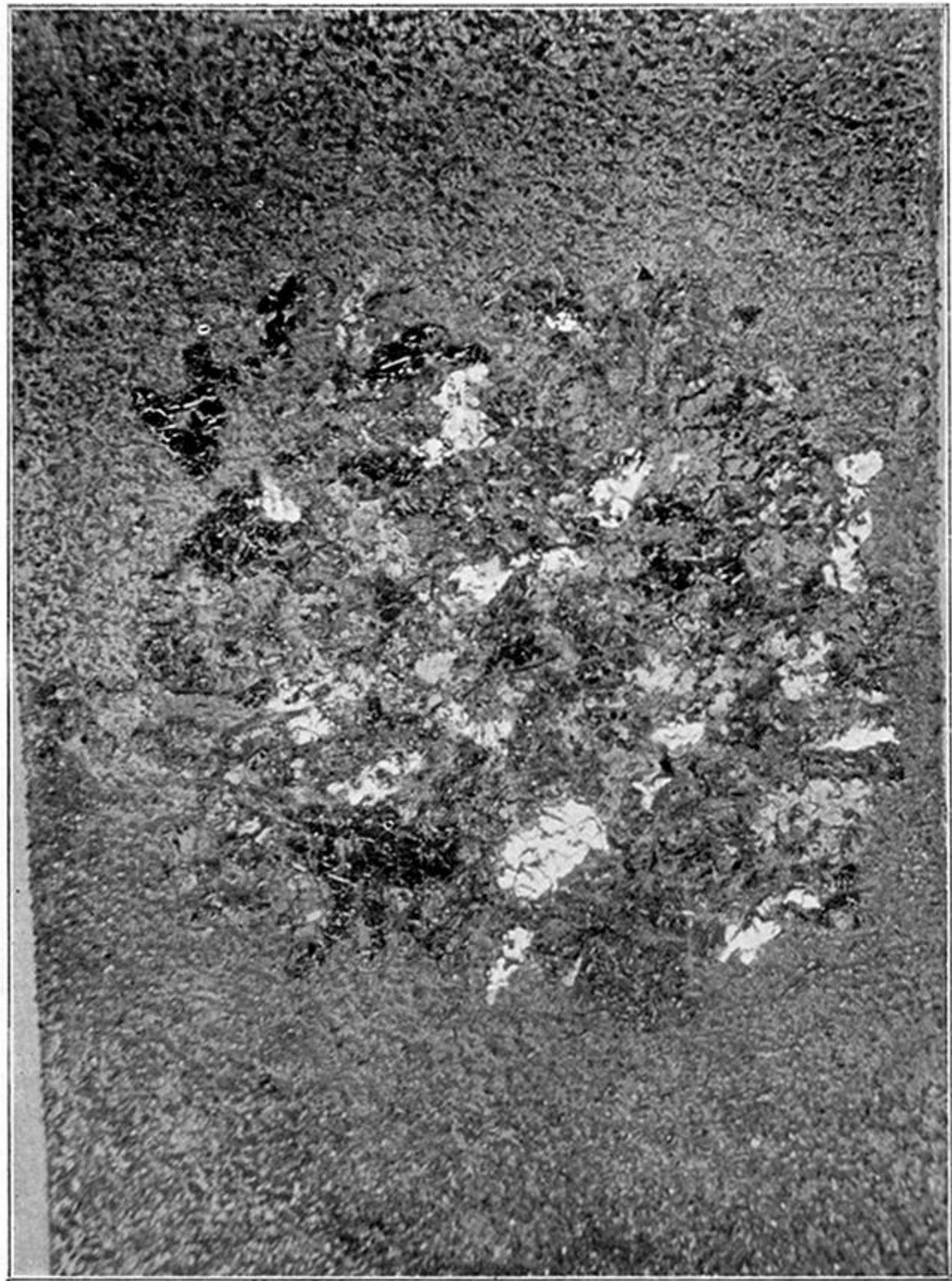
Fig. 10. Strained crystal, re-etched \times 6 .
