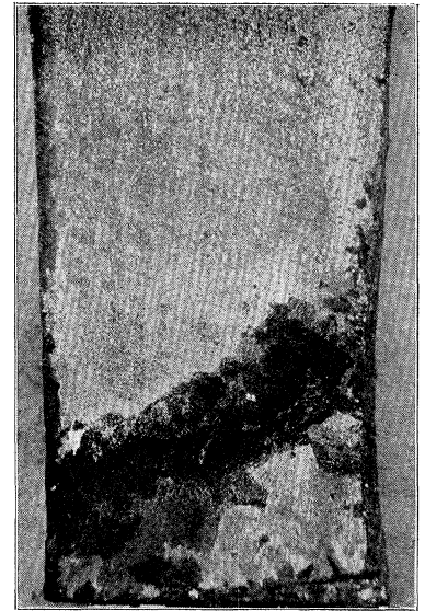
Fig. 22. A single crystal after straining in tension and re-etching \times 4 .
