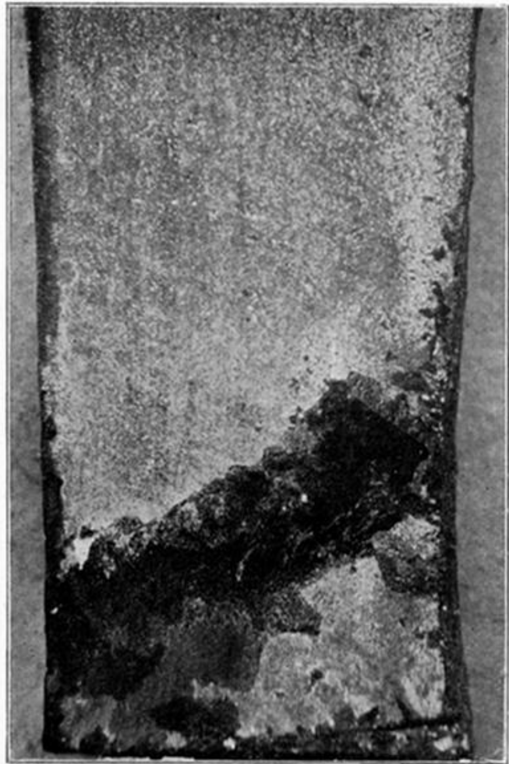
Fig. 22. A single crystal after strain- ing in tension and re-etching \times 4 .
