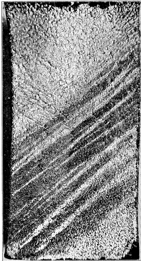
Fig. 20. A single crystal after straining in tension and re-etching \times 5 .
