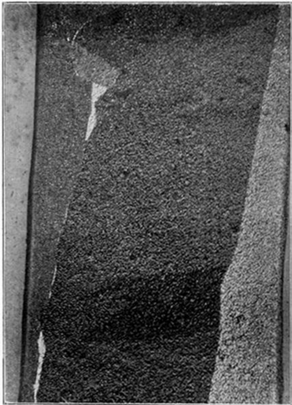
Fig. 24. A single crystal after strain- ing in tension, cooking 2 hours at 100^{\circ} C., and re-etching.
